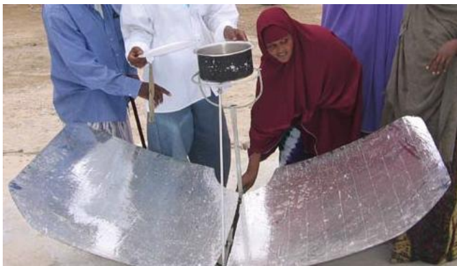
Photo credit: Jim Lindsay, Sunfire. This is a 'butterfly' parabolic solar cooker comparable in design to the majority of those in Tibet
