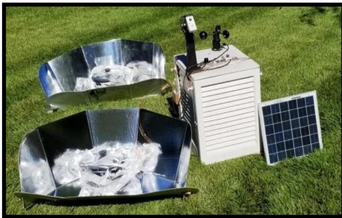
Testing the power of Cookits using a Stevenson box, two pyranometers and an anemometer, powered by a solar panel.
