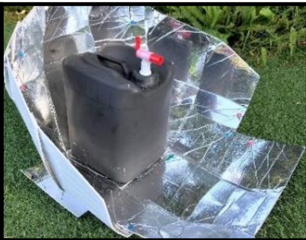
The Haines 2 can pasteurize a 5-gallon jerrican of water in under four hours.
