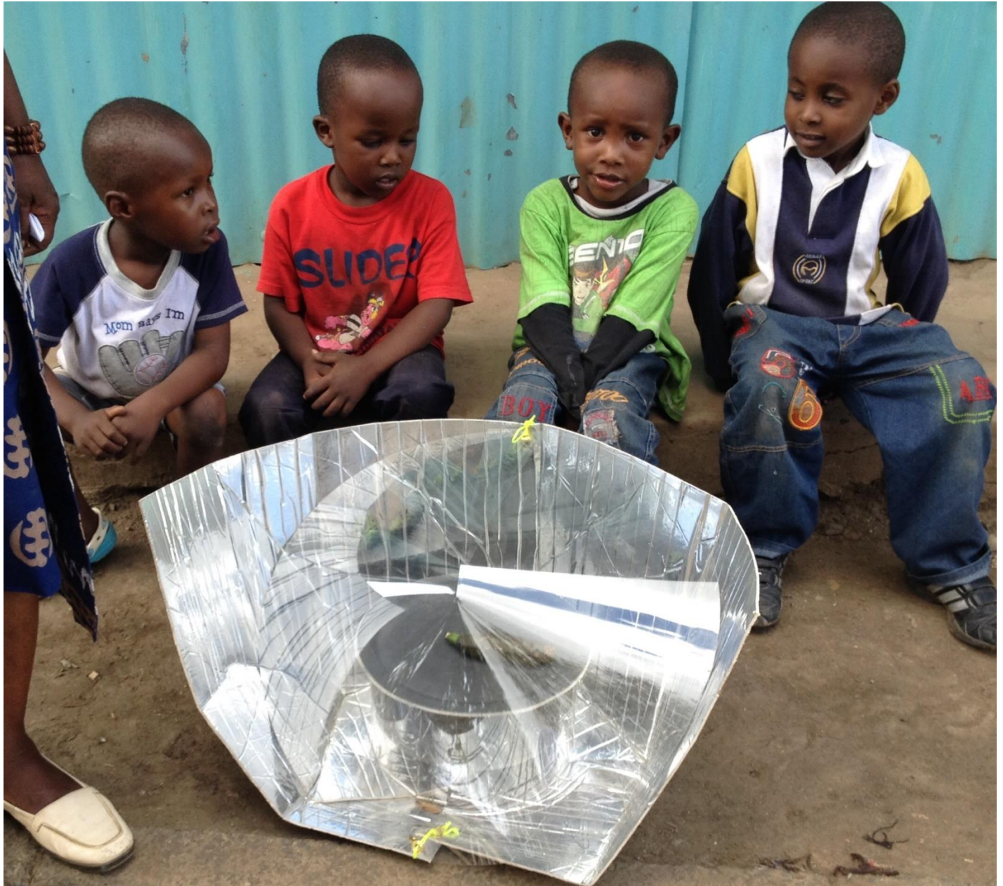
The Haines solar cooker is an affordable yet durable solar cooker that holds promise for Chad refugee camps. It is currently being tested in Chad.
