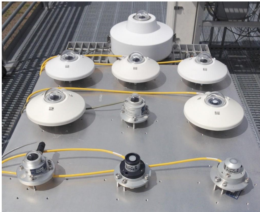
Figure 1. Examples of pyranometers at the US National Renewable Energy Laboratory.
