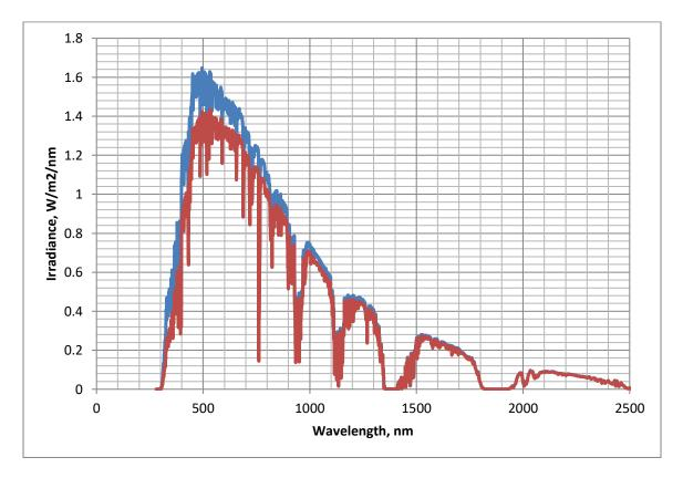
The figure above shows the ASTM G173-03 reference solar spectra for global tilted sensors (blue) and direct radiation within 2.5 degrees of the sun (red). The visible spectrum runs from about 400 nm to 700 nm.
