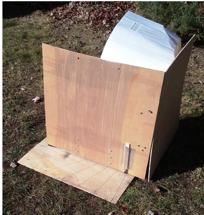
Figure 2. Rig for measuring vertical directivity
