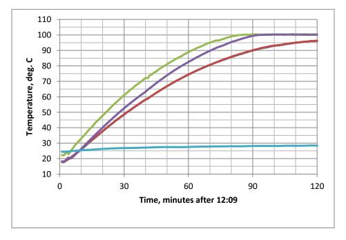
Green – large Yajad Italian pot, sealed watertight with metal tape, in sleeve, reflector #2 Purple – Haines Dutch oven #3 in sleeve, reflector #3 Red – Duracera blue pot, unsealed, with sleeve and Haines #1 lid in reflector #1
