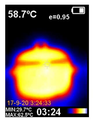
The heat loss is higher where the pot is cooler (red on this color scale). (The pot's outline is red because emissivity at near-grazing angles is reduced for most nonmetallic materials).
