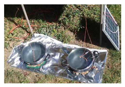
Two thermocouples were placed in the pots for redundancy. The comparison showed that the sealed pot was about 5 deg. C hotter than the unsealed pot after 1 hour. Although temperature differences may vary, the general conclusion is that a sealed pot is better than an unsealed pot.
