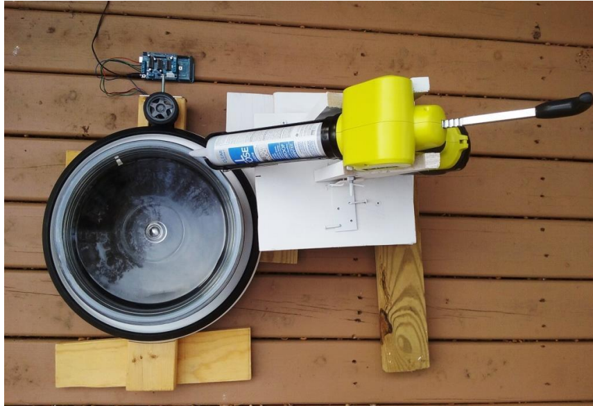
Figure 3. Arrangement of caulking gun and turntable with HotPot mounted, top view.
