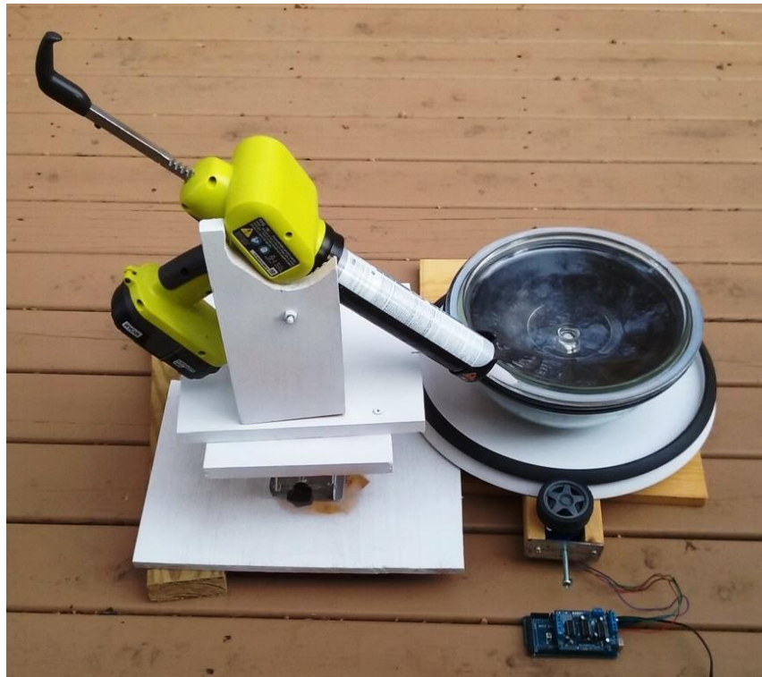
Figure 2. Arrangement of caulking gun and turntable with HotPot mounted, side view.
