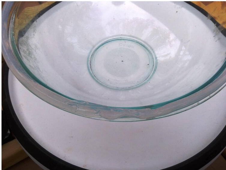
Figure 6 above shows a thin spot at the ends of the liner gasket. An effort to smooth this out manually was not successful.
