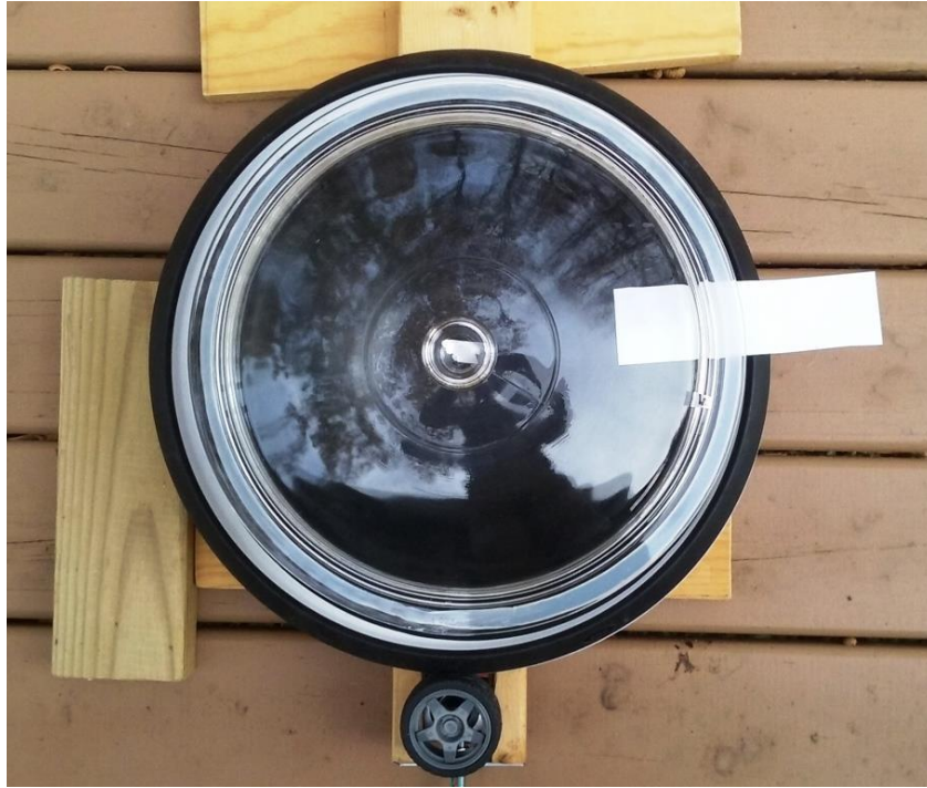
Figure 6. HotPot lid with new silicone gasket, resting on HotPot metal bowl. A strip of paper could pass easily through the gap.
