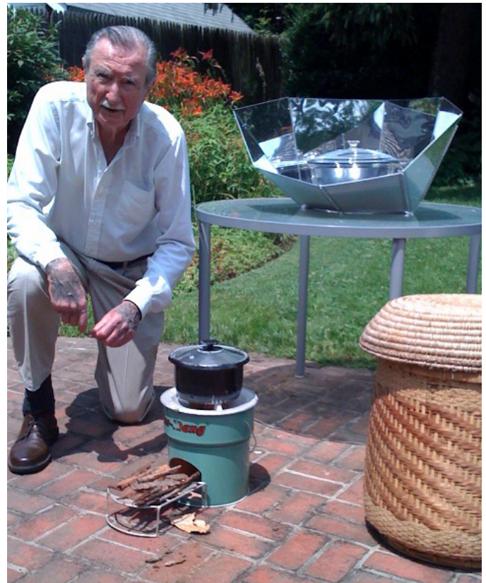
SHE board member and co-founder Darwin Curtis displays the three components of the "integrated cooking" system: A fuel-efficient stove (requiring only small pieces of wood, as shown), a retained heat device (the large basket) and a solar oven (in this example, a HotPot, sitting on table).
