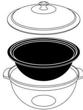
Figure 1. Three components of the HotPot solar cooker vessel
