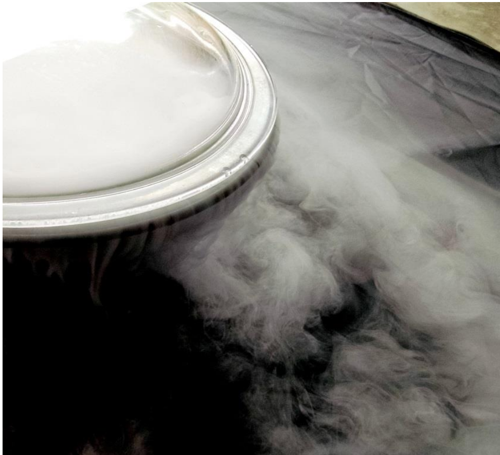
Figure 3. Water vapor escaping from lid gap.
