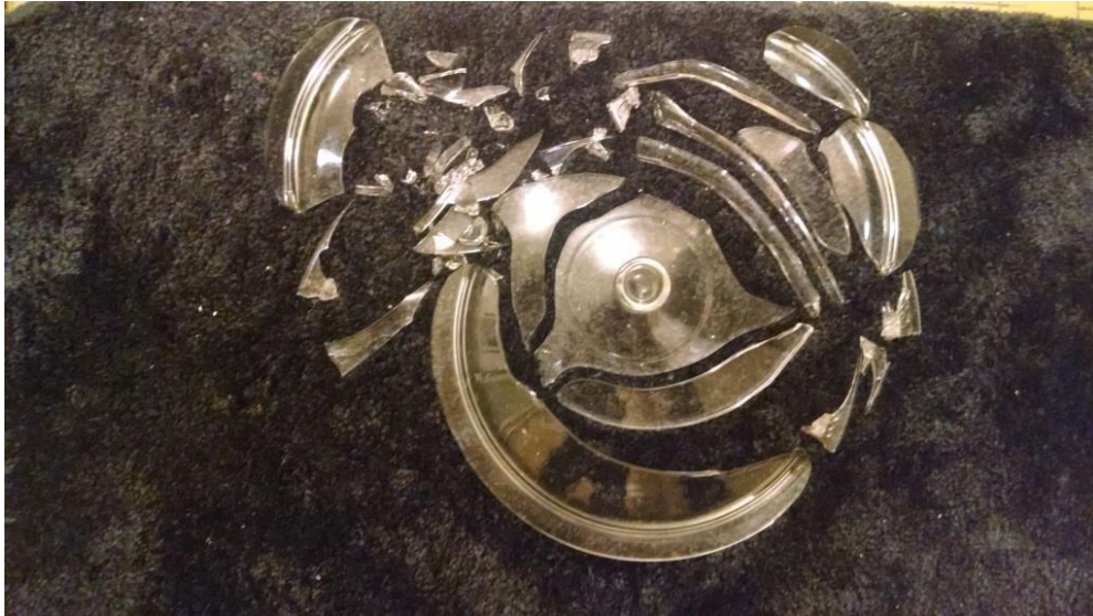
Figure 4. Shattered lid of the HotPot after drilling.
