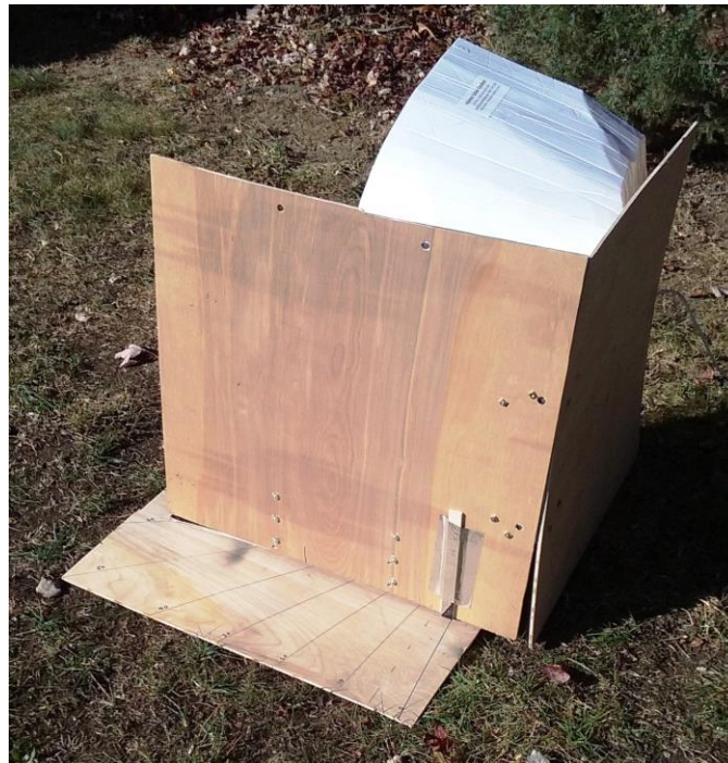
Figure 2. Rig for measuring vertical directivity
