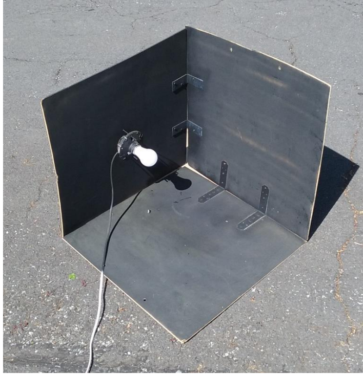
Figure 3. Rig for measuring bare bulb directivity.
