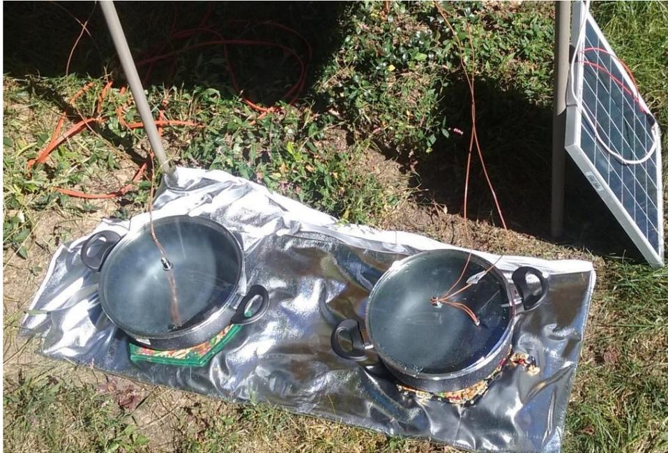
Two thermocouples were placed in the pots for redundancy. The comparison showed that the sealed pot was about 5 deg. C hotter than the unsealed pot after 1 hour. Although temperature differences may vary, the general conclusion is that a sealed pot is better than an unsealed pot.
