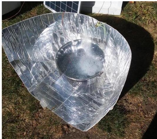
The small sealed Yahad pot performed almost the same as the Haines Dutch oven (which has a tight silicone rubber lid seal). Both of these came to a full boil after 100 minutes.
