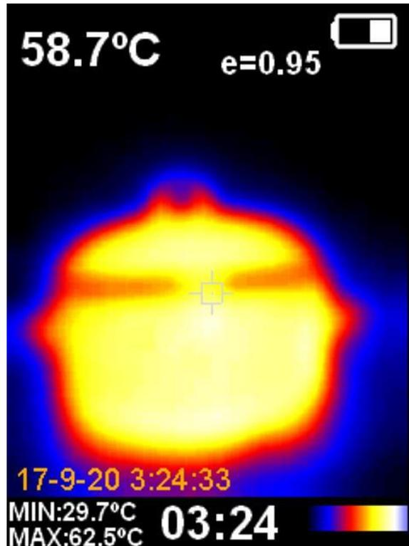
The heat loss is higher where the pot is cooler (red on this color scale). (The pot's outline is red because emissivity at near-grazing angles is reduced for most nonmetallic materials).
