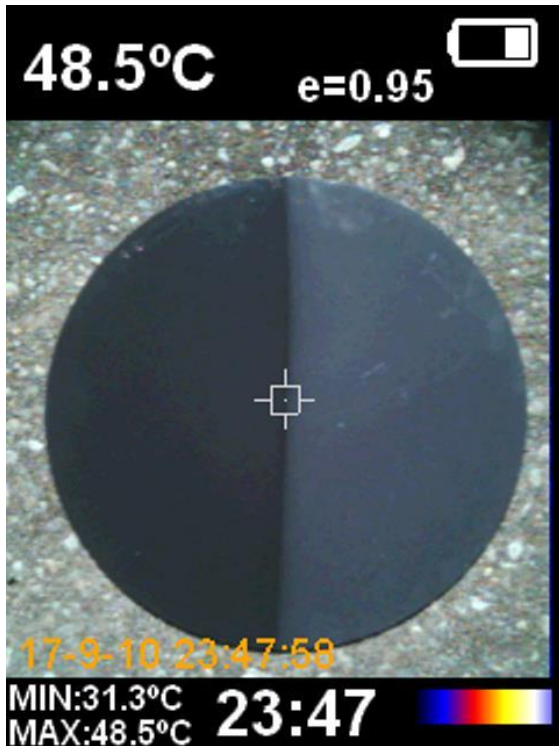
Figure 3 - This is a closeup of the first disk which is half Krylon Ultra-Black (left half) and half Rust-Oleum stove paint. This is the image in visible light. The Ultra-Black paint has an emissivity of 0.96 (or reflectivity of 0.04) from 2 to 5 microns and 0.95 from 8.5 to 14 microns, according to the NASA reference data.
