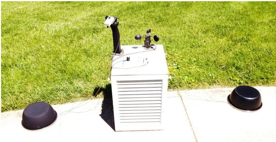
Figure 6. Experimental setup to compare performance of two types of paint; the Ultra-Black painted pot is on the left.
