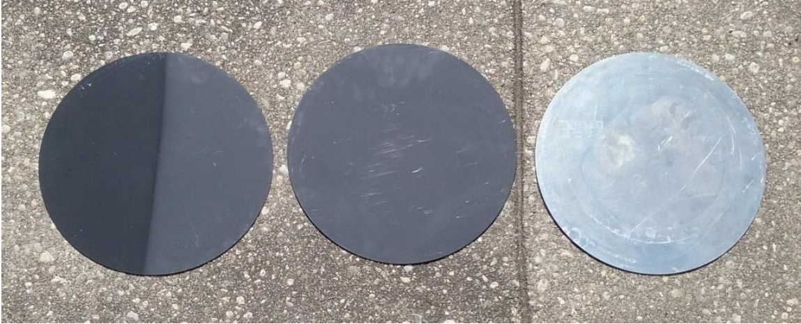
Figure 1 –The test items were three aluminum disks, each 12 in. (30 cm) diameter, 0.06 in. (0.15 cm) thick. These were set flat on a concrete sidewalk in clear sun and allowed to heat to equilibrium (over 15 minutes). The disk on the left is painted on the left half with Krylon Ultra-Black 1602 spray paint (see Appendix for sources). The other half is painted with Rust-Oleum High Heat stove paint. The middle disk is painted entirely with the High Heat stove paint. The right disk is bare unpolished aluminum.
